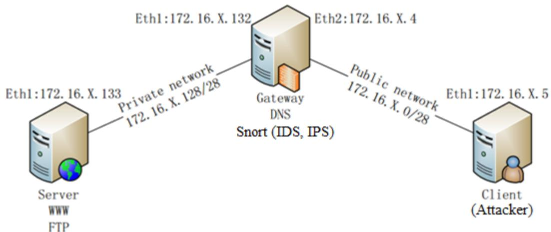
Install Snort package on your gateway and run another internal computer accessing the external network through the gateway. Configure iptables properly on the gateway to allow traffic from vnet 1 to vnet 2 and vice versa.. Please follow the steps below to install Snort in your Gateway:
