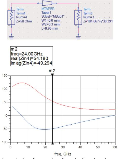
The tapered transformer transformed the impedance from  $Z_{RX} = 104.667+38.391$  j Ohm to 54.18-49.294 j Ohm.
