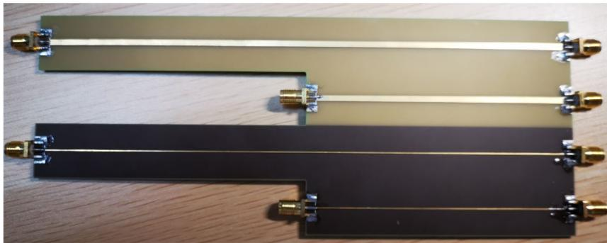
Impedance traces, the first 20cm trace is used in this example
