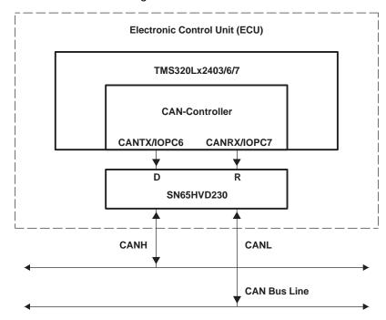
Figure 36. Details of a Typical CAN Node
