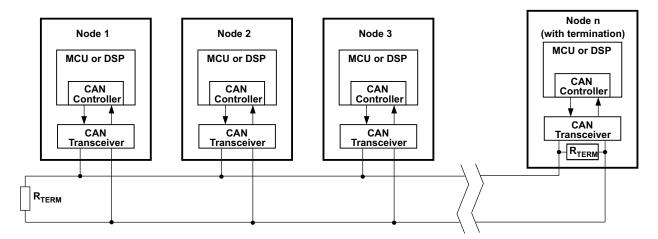
Figure 38. Typical CAN Bus
