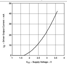
Figure 15. Driver Output Current vs Supply Voltage
