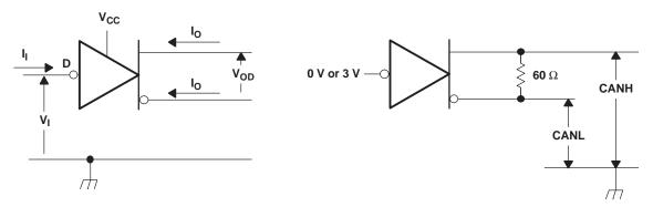
Figure 18. Driver Voltage and Current Definitions
