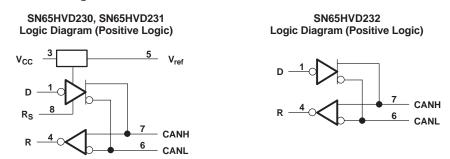
Figure 29. Logic Diagram (Positive Logic)
