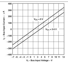
Figure 3. Bus Input Current vs Bus Input Voltage
