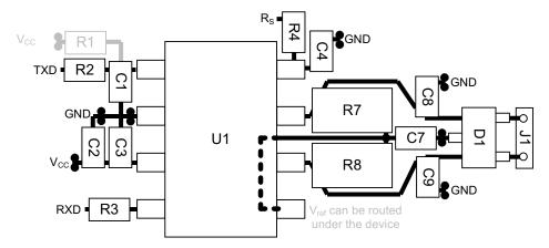
Figure 44. SN65HVD23x Board Layout
