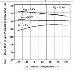
Figure 12. Driver High-to-Low Propagation Delay Time vs Free-Air Temperature
