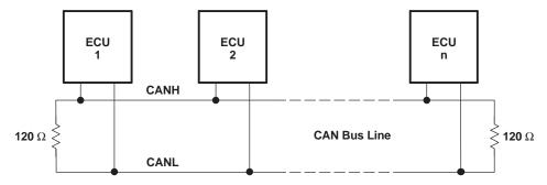
Figure 37. Typical CAN Network
