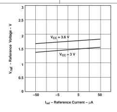
Figure 17. Reference Voltage vs Reference Current
