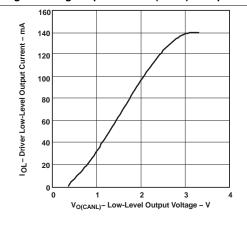
Figure 4. Driver Low-Level Output Current vs Low-Level
