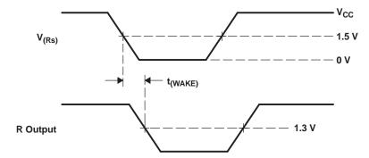
Figure 25.  $t_{(WAKE)}$  Test Circuit and Voltage Waveforms
