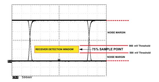
Figure 42. Typical SN65HVD230 Differential Output Voltage Waveform
