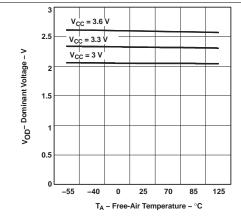
Figure 6. Dominant Voltage ( $V_{OD}$ ) vs Free-Air Temperature
