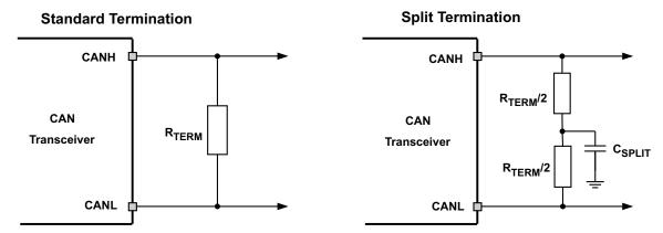
Figure 39. CAN Bus Termination Concepts
