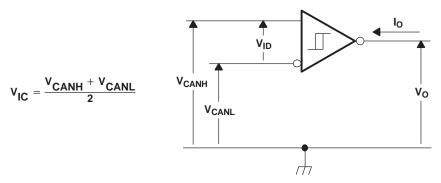
Figure 22. Receiver Voltage and Current Definitions
