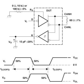
A. All  $V_1$  input pulses are supplied by a generator having the following characteristics:  $t_r$  or  $t_f \le 6$  ns, Pulse Repetition Rate (PRR) = 125 kHz, 50% duty cycle.
