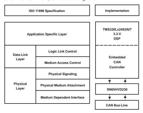
Figure 28. Layered ISO 11898 Standard Architecture
