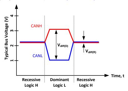
Figure 34. CAN Bus States (Physical Bit Representation)
