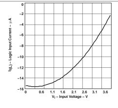
Figure 2. Logic Input Current (Pin D) vs Input Voltage
