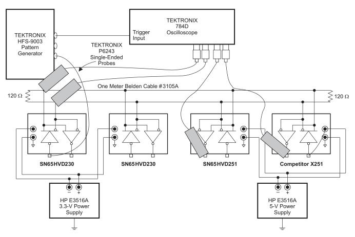
Figure 43. 3.3-V and 5-V CAN Transceiver System Testing
