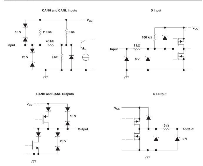
Figure 27. Equivalent Input and Output Schematic Diagrams
