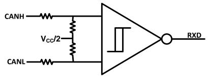
Figure 35. Simplified Recessive Common Mode Bias and Receiver
