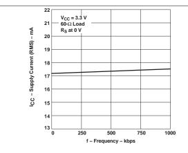
Figure 1. Supply Current (RMS) vs Frequency
