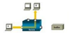
With a LAN switch, traffic travels point-to-point only; packets no longer replicated; network visibility is lost
