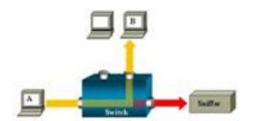
SPAN (or mirroring) port was invented to replicate packets of a single port or a single VLAN for monitoring
