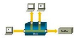
In the past, with a shared hub, packets are replicated on all ports; plug a "sniffer" into any data port will see all traffic!!
