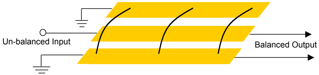
Figure 7 Coupled line balun using multiple coupled lines
