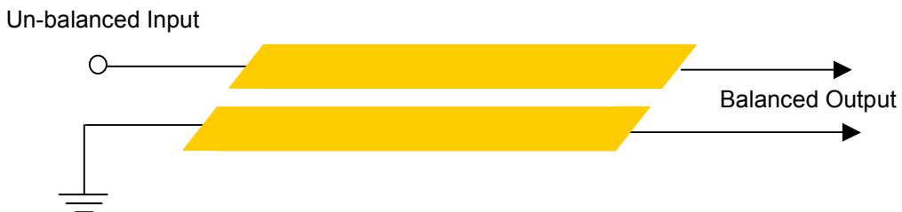
Figure 6 Simple coupled line balun
